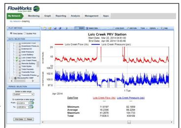
FlowWorks Reporting showed a significant main break that was identified and repaired within a four day window, and shows how a 2 psi adjustment of the Louis Creek PRV settings saved approximately 8 GPM in system losses.
